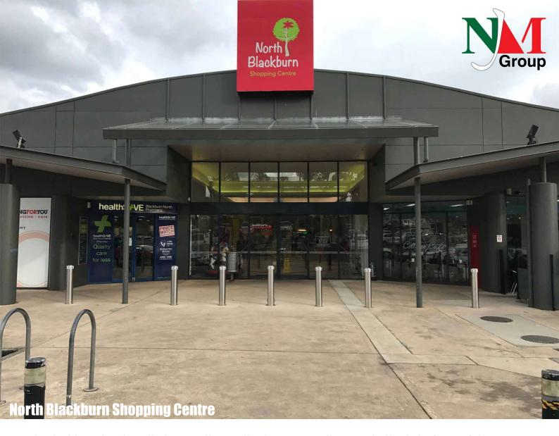
North Blackburn has installed Australian Bollards' 168mm diameter bollards in front of the entrance. The sub surface mounted, concrete backfilled bollards prevent ram-raids while allowing authorised vehicles to easily pass anytime, as the center bollard is removable.
